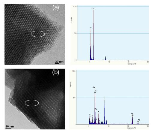
Fig. 3. HRTEM images of samples: (a) SBA-15 and (b) 51SVO/SBA-15.
