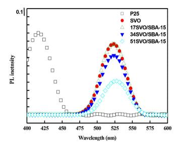
Fig. 5. Normalized PL intensity of the samples measured at 300 K.
