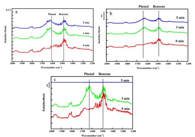
Fig. 4. Time-dependent DRIFT spectra of adsorbed benzene and phenol on various samples during the visible-light irradiation: (a) P25, (b) SVO, and (c) 51SVO/SBA-15.
