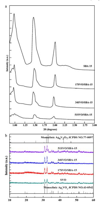
**Fig. 1.** (a) Low angle XRD patterns of SVO and SVO/SBA-15; (b) wide angle XRD patterns of SVO and SVO/SBA-15.
