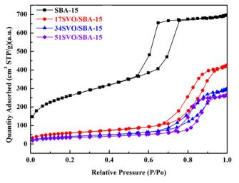
**Fig. 2.** N<sub>2</sub> adsorption–desorption isotherms of SBA-15 and SVO/SBA-15 samples.
